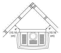
Figure 4 - Clearance for Corner Installation
